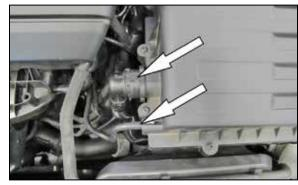
3. Disconnect the secondary air tube and vacuum hose from the air filter housing.
