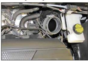
12. Install one of the provided coupling hoses (08185) onto the turbo inlet and secure with the provided hose clamp.
