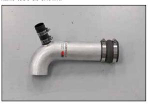
16. Install the remaining coupling hose (08185) onto the K&N® intake tube as shown.
