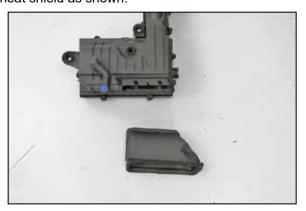
9. Remove the fresh air intake scoop from the factory air filter housing.
