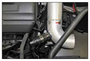
19. Connect the secondary air hose onto the Quick disconnect fitting and connect the vacuum line to the fitting installed into the K&N® intake tube.
