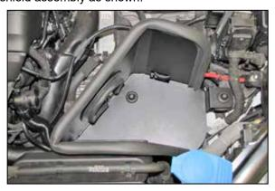
11. Install the heat shield assembly onto the factory air filter housing mounting studs.
