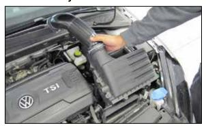
4. Lift up the air filter housing to dislodge it from the mounting grommets and then rotate the assembly up from the rear to disengage it from the fresh air intake and remove it from the vehicle.
