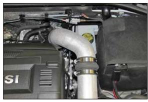
18. Install the rear K&N® intake tube into the coupling hose on the front intake tube and then into the coupling hose at the turbo inlet, adjust the tubes for best fit and then secure with the provided hose clamps.
